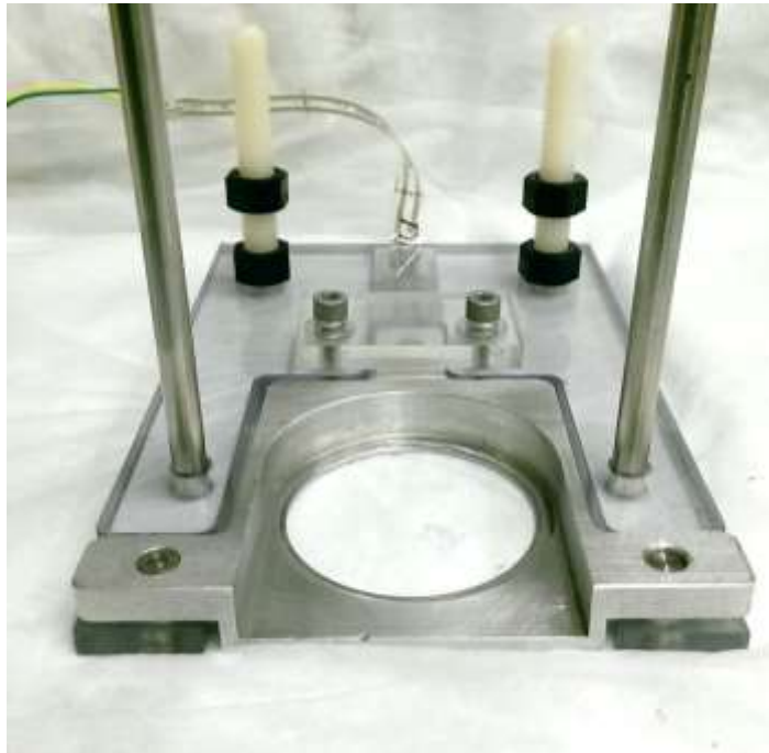
Figure 46: Image of force sensor plate mounted in device base
