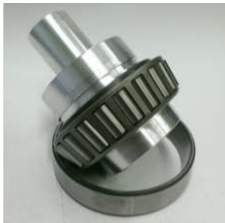
Figure 10: Cone press-fit into tapered roller bearing
