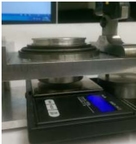
Figure 20: Cone lowered onto laboratory scale to detect force upon contact
