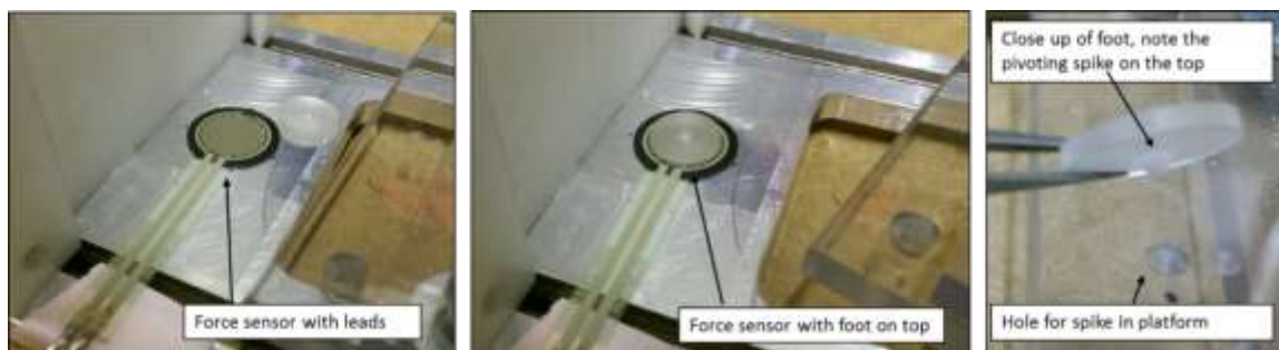
Figure 23: Resistive Load sensor with PDMS rubber spacer and sensor foot with pivot spike
