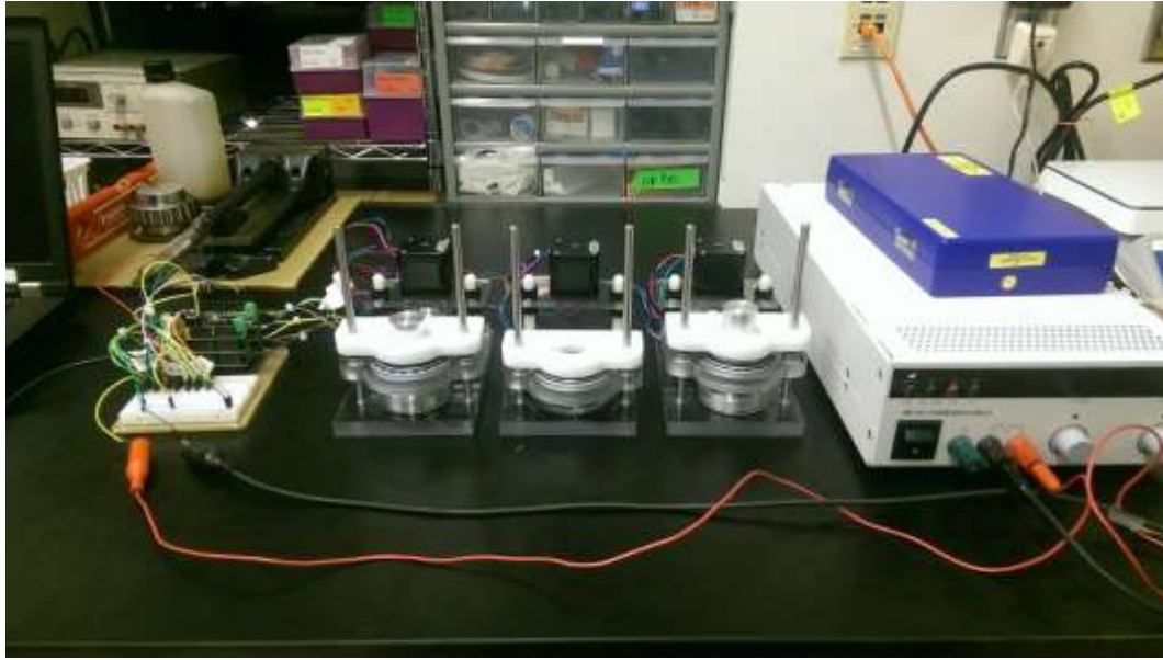
Figure 41: Cone and plate flow system with 3 devices, motor controllers, drives, and power supply
