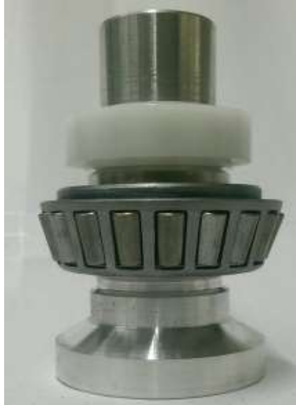
Figure 43: Image of cone and bearing assembly with primary tapered bearing and secondary stabilizing bearing (white)
