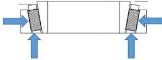
Figure 11: Side view cut-away of 2" diameter steel tapered roller bearing with arrows representing reaction forces to indicate constrained directions
