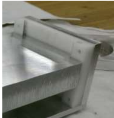
Figure 26: Dovetail rail of carriage plate and vertical rail of Teflon upright
