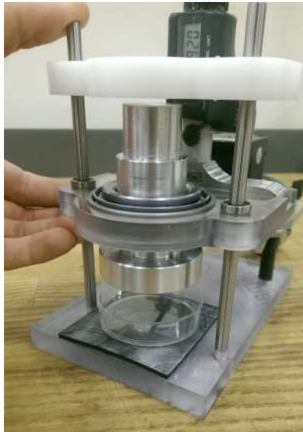
Figure 47: Expanded view demonstrating the sliding linear bearings and carriage plate
