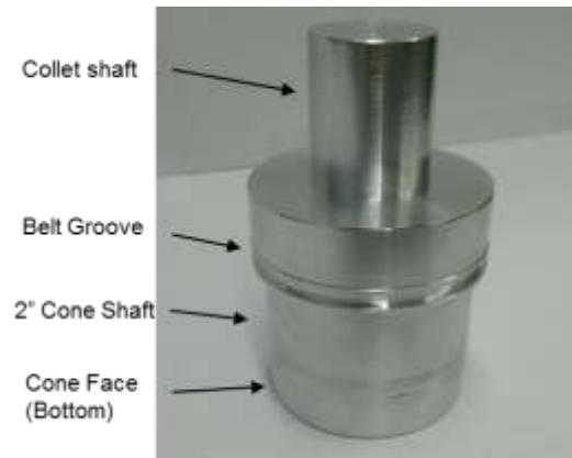
Figure 9: Cone with 1" collet shaft for mounting in lathe chuck
