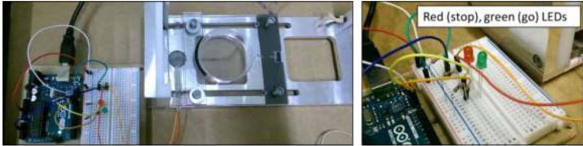
Figure 24: Sensor plate electronics assembly with LED indicator lights
