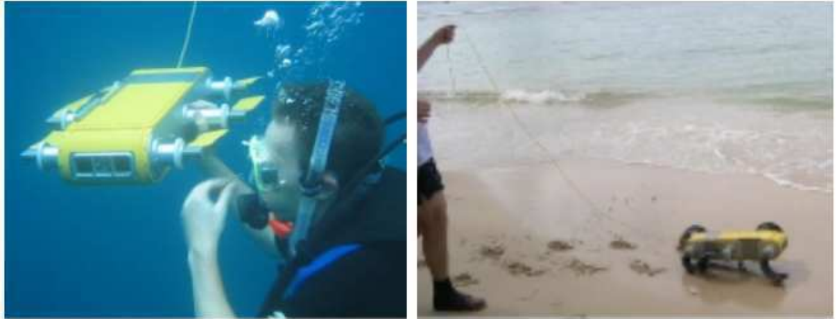
Figure 2.3. An amphibious robot using stereo cameras
