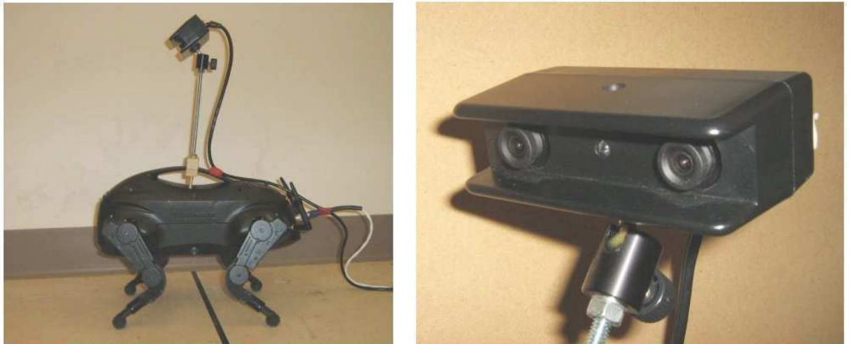
Figure 2.4. LittleDog and the stereo camera setup [49]
