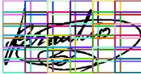
Figure 3.3: Cartesian 6x6 20% overlapping grids shown altogether.
