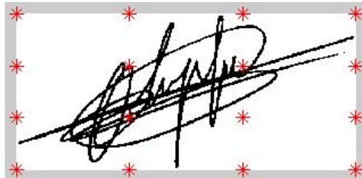
Figure 3.6: Origin points selection pattern for log-polar coordinates.
