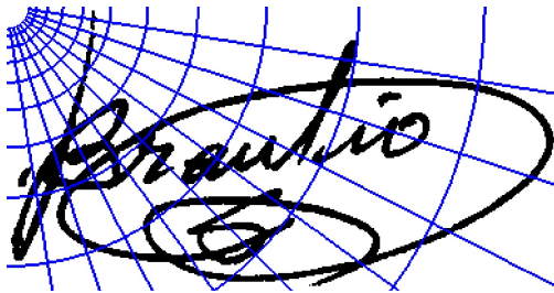
Figure 3.5: Log-polar grids, origin taken as the top-left corner.
