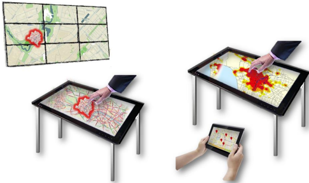
Figure 2.3: Example of a multi-display overview + detail interface [1]
