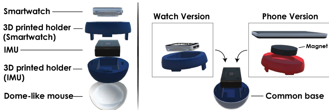
Figure 4.9: Arrangement of TDome elements for the Small version (left). Both TDome versions are rapidly interchangeable (right).
