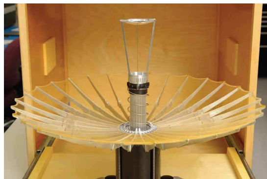
Fig. 10. Deployable reflectors for CubeSats.
