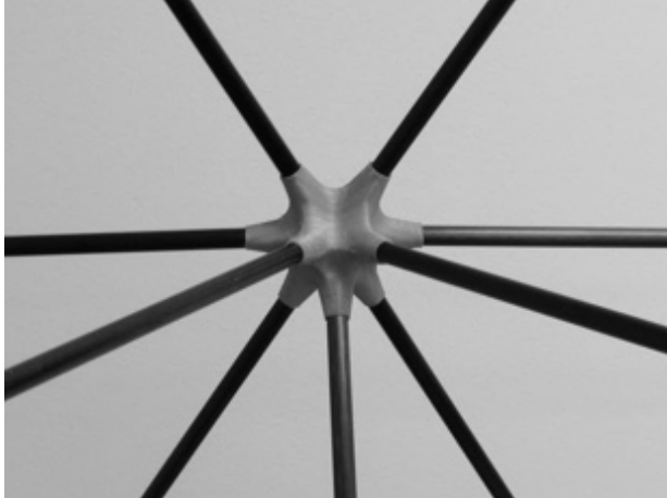
Figure 41. Prototype 3D-Printed Optimized Joint. Use of 3D-printing techniques with a highly dexterous print head can enable fabrication of joints optimized for the service loads, maximizing structural efficiency.
