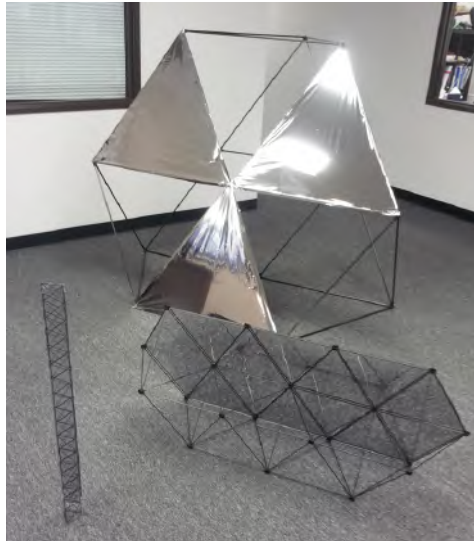
Figure 49. Testing methods for attaching membranes and other components to support structures. We built tetrahedral truss sections out of pultruded carbon fiber tubes and 3D-printed plastic joints, to provide test beds for methods of attaching surface elements.
