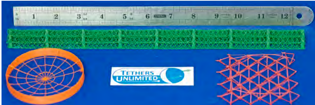
Figure 2. Samples fabricated using FFM. On Earth, slumping due to gravity limits the element dimensions of sparse structures to centimeter scales, but this limit will not be present in microgravity.
