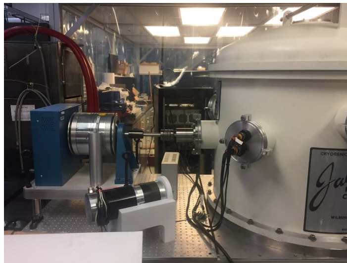
Figure 4: Magtrol Dynamometer, Cryo-mech Chamber, and UUT Power Feedthrough
