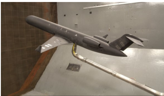
Fig. 5 The GTT is shown mounted in the 12-Foot LST. The elevator and rudder surface arrangement is visible.
