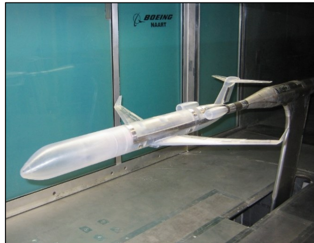
Fig. 11 The GTT configuration is shown mounted in the BR&T NAART.
