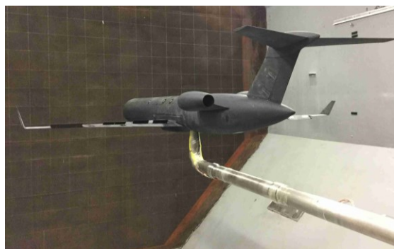
Fig. 6 The GTT is shown mounted in the 12-Foot LST on a bent sting mount. The arrangement of the roll control surfaces (aileron and spoilers) is visible on the left wing.
