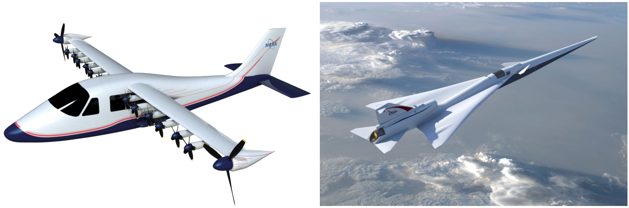
(a) X-57 Maxwell electric aircraft with leading edge distributed propulsion. 31,32 (b) Rendering of the Quiet Supersonic Transport (QueSST). k
