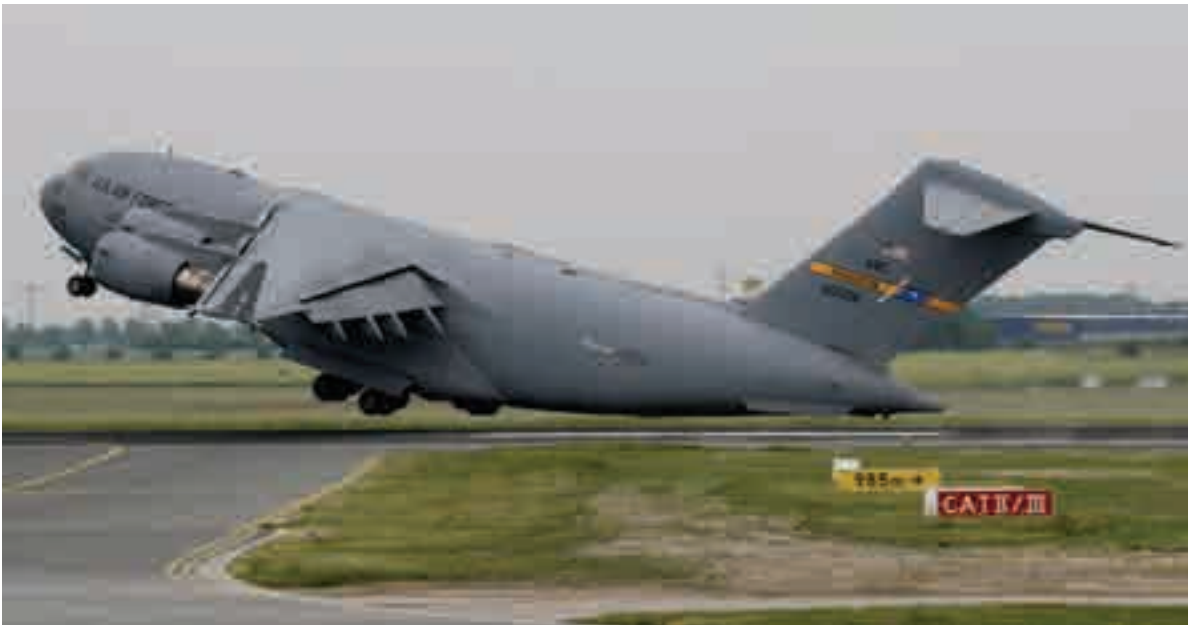
Fig. 1-24. The Boeing C-17A, a STOL transport powered with gas turbines. Jet engine exhaust increases lift from the flaps.
