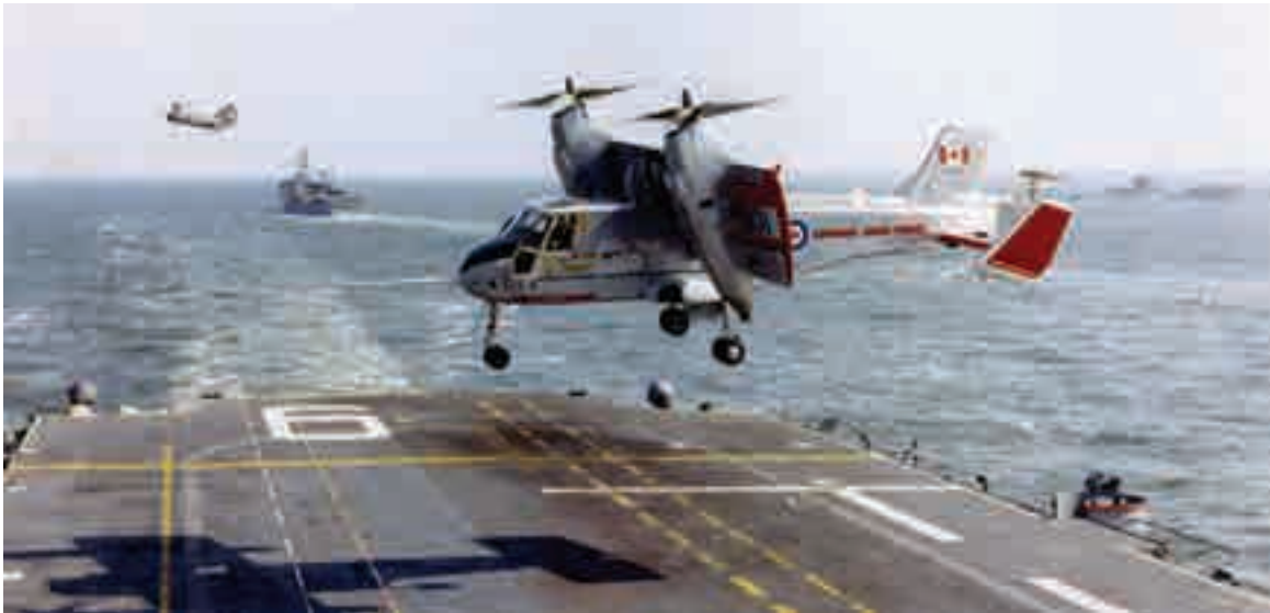
Fig. 2-86. The Canadair CL-84. This 10,600-pound VTOL technology demonstrator made its first hovering flight on May 7, 1965. The first full conversion back and forth from hover was made on January 17, 1968. The CL-84's success far exceeded either Vertol's VZ-2 or Hiller's X-18.
