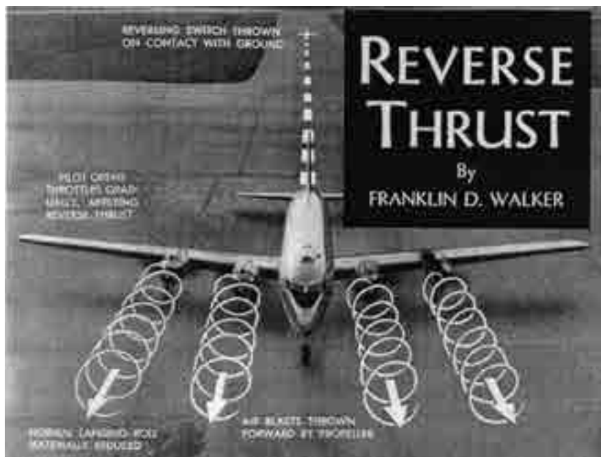
Fig. H-2. The caption of this artist's rendition reads, "Picture illustrates effect of reverse thrust in reducing landing roll. Churning props throw air forward, brakes plane."
