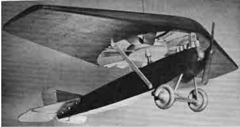
Fig. 1-17. Jacob Ellehammer believed that “an aircraft should have the maximum cruising speed and require a minimum of runway.” A venetian blind was to unroll over the fans (top and bottom) in forward flight [20].
