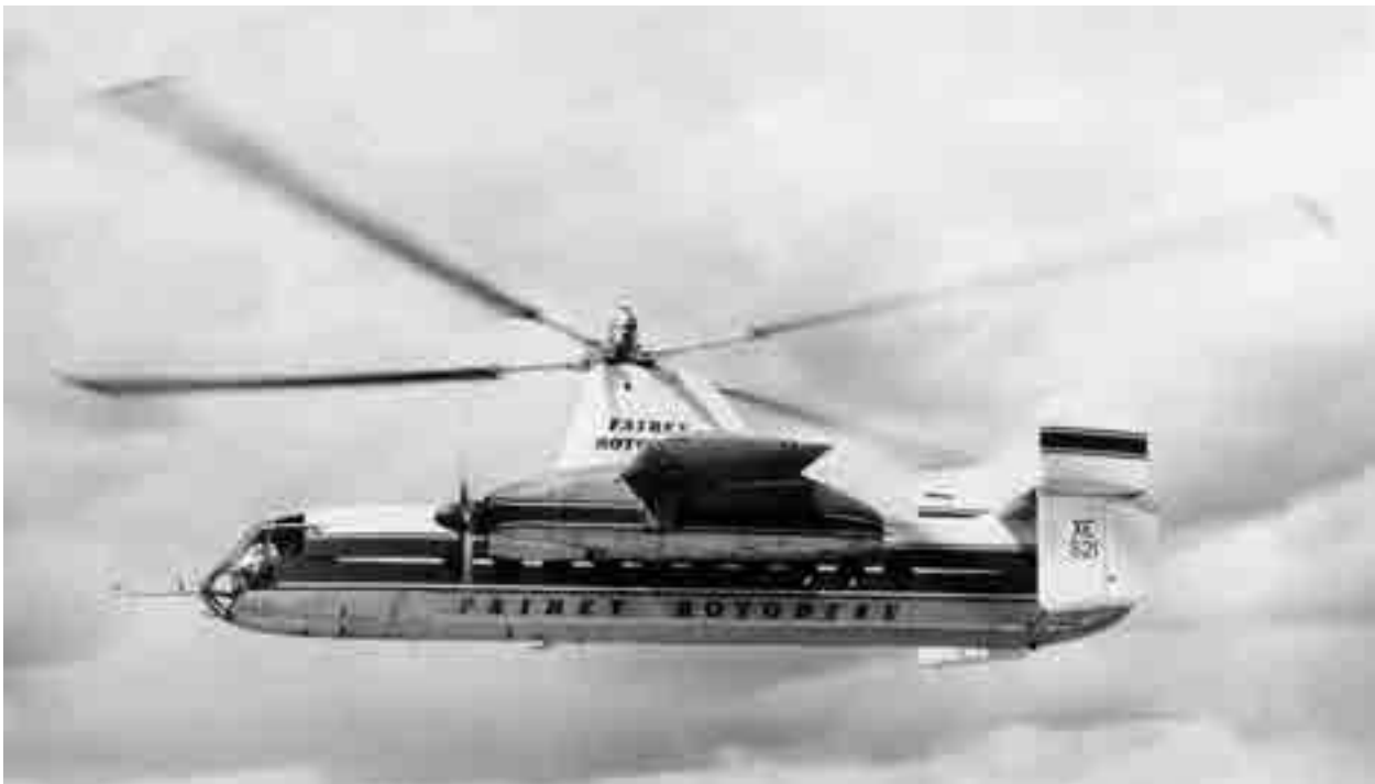
Fig. 2-7. The Rotodyne first flew on November 6, 1957. On January 5, 1959, it raised the world speed record to 167 knots [70].
