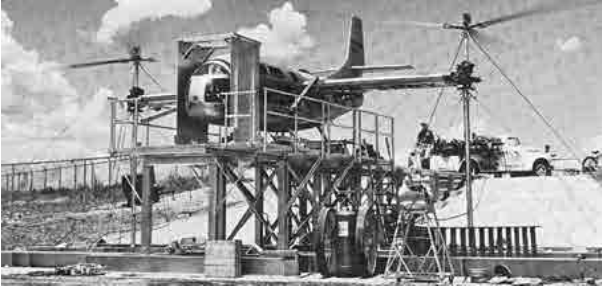
Fig. F-1. Ground tests to develop a stable rotor-pylon (from Bob Lynn's 1992 Nikolsky Lecture).
