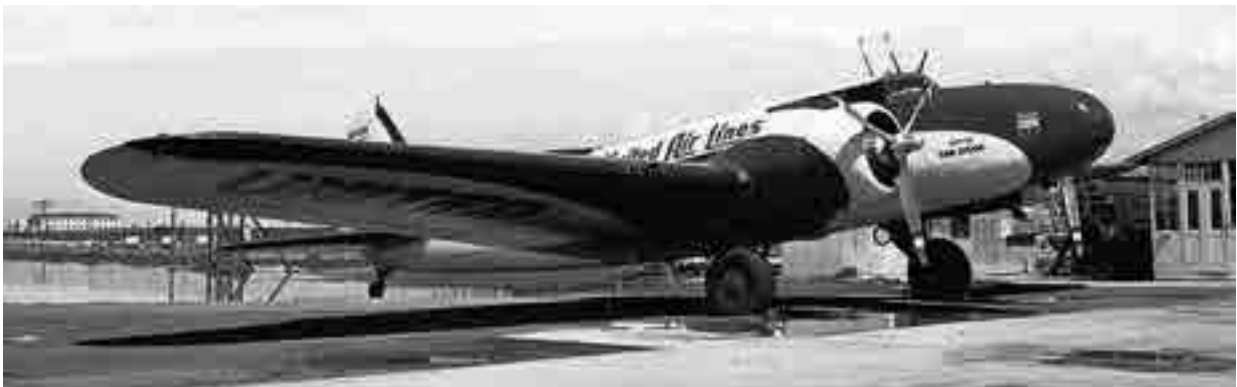
Fig. 3-201. The Boeing Model 247, a 10-passenger airliner, overcame many of the trimotor's problems so that the airlines could make a profit carrying passengers only. Its first flight was on February 8, 1933.
