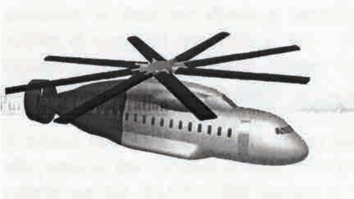
Fig. 2-199. Suppose you accept, say, eight blades attached to a hingeless hub, forget the wing, and operate the rotor at high speed at an advance ratio of 1.5 or higher. A Sikorsky paper [79] got me thinking.
