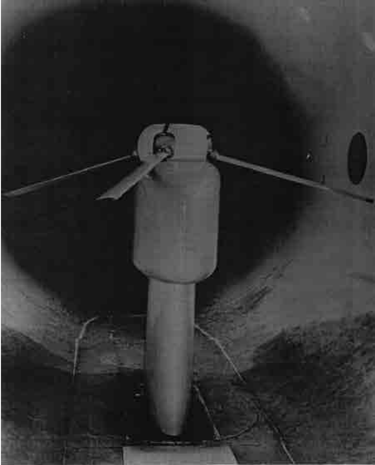
Fig. 2-16. The Fairchild 8-foot-diameter RVR as installed in the NASA Ames 12-foot pressure wind tunnel [77]. The rotor solidity was 0.1333.
