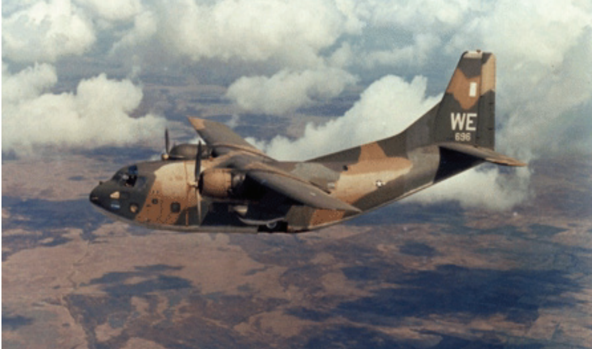
Fig. 3-142. The Fairchild C-123B Provider had a maximum takeoff gross weight of 60,000 pounds [564-569].
