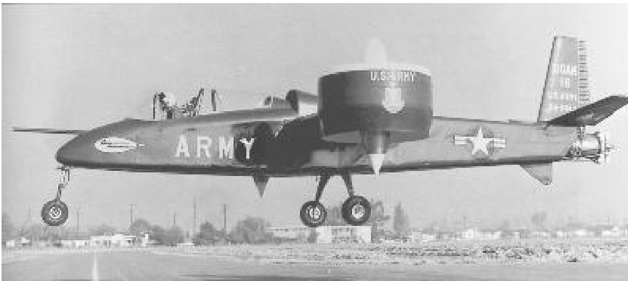
Fig. 2-128. The Doak VZ-4A made its first flight on February 25, 1958. This 3,200-pound aircraft was initially powered with an 840-horsepower Lycoming YT-53 turboshaft engine, which was later upgraded to a 1,000-horsepower YT-53A.
