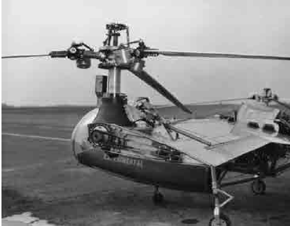
Fig. 2-117. The screw jack conversion actuator assembly of the first tiltrotor, the Transcendental Model 1 (photo courtesy of Howard Levy and Mike Hirschberg).
