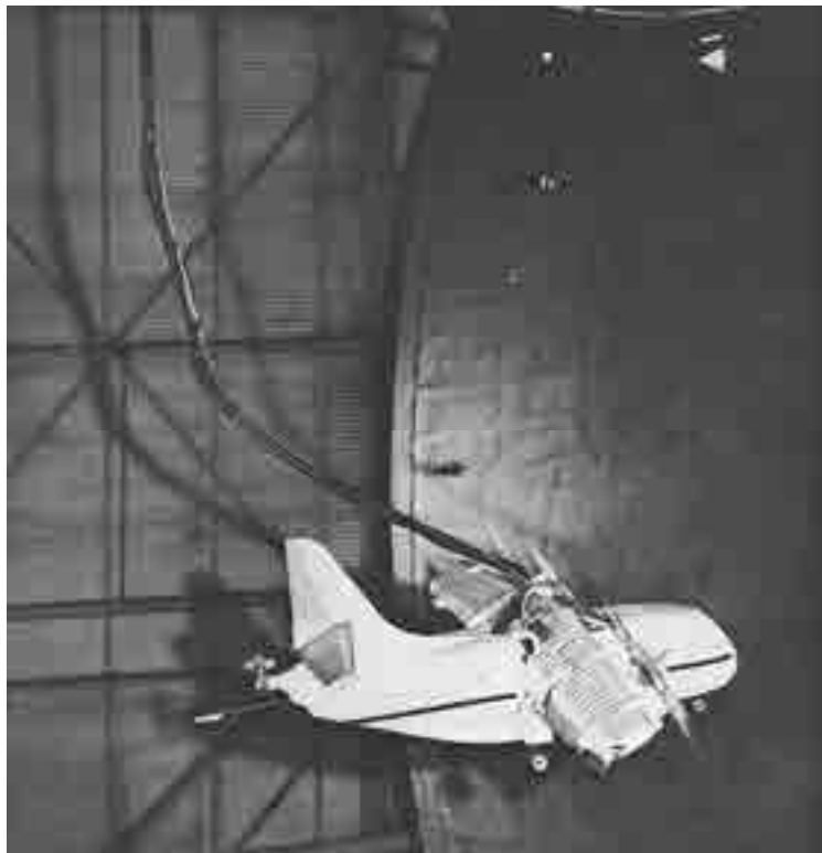
Fig. 2-109. The 0.11-scale model with a wingspan of 7.5 feet was tested in "free flight" in the Langley 30- by 60-foot wind tunnel [223].
