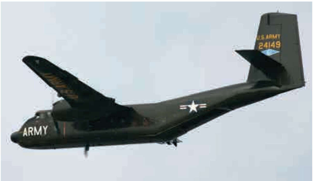
Fig. 3-143. The de Havilland of Canada CV-2B Caribou had a maximum takeoff gross weight of 28,500 pounds [495-498, 502, 505, 570].
