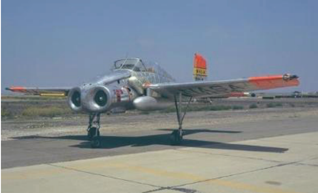
Fig. 2-129. Larry Bell’s Bell Aircraft Corporation became Bell Aerospace in 1965. The company obtained a contract for the X-14 in July of 1955. This 4,270-pound aircraft was initially powered by two Armstrong Siddeley ASV8 Viper turbojet engines slung under the nose and exhausting through vane cascades beneath mid-fuselage. Each Viper was rated at 1,750 pounds thrust. It first hovered on February 17, 1957.
