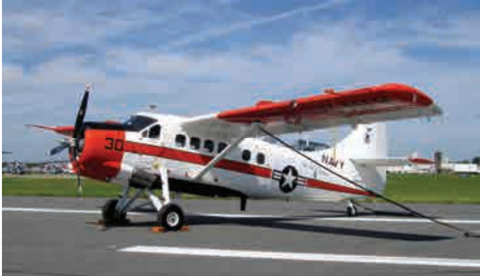
Fig. 3-162. The de Havilland DHC-3 Otter was bought by all the U.S. services. This 8,000-pound aircraft was powered by a 600 bph P&W piston R-1340-S1H2-G engine. It could cruise economically at 120 knots at 5,000 feet. It's first flight was on December 12, 1951, and the aircraft continued de Havilland of Canada's reputation for rugged STOL performance [495, 504, 604].
