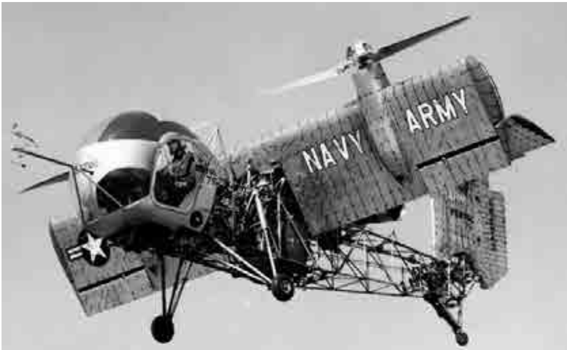
Fig. 2-78. The Vertol VZ-2 tiltwing. This 3,500-pound VTOL technology demonstrator, piloted by Leonard Lavassar, made its first hovering flight on August 13, 1957. The first full conversion back and forth from hover was made on July 15, 1958.
