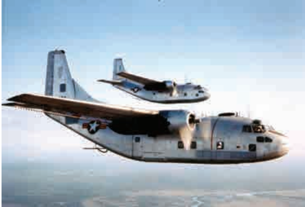
Fig. 3-9. The Fairchild C-123 logistical transport was modeled at 0.4 scale by the N.A.C.A. as the baseline for STOL research.
