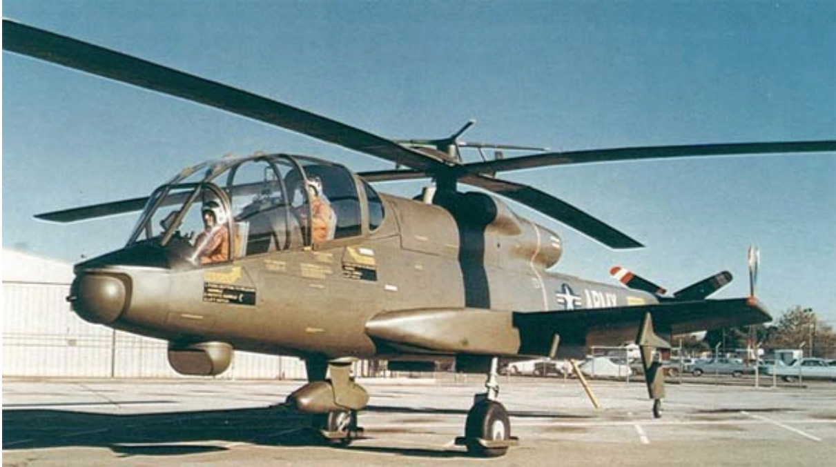
Fig. 2-45. The Lockheed AH-56 had a tail rotor for hover, and a pusher propeller and wing for forward flight.
