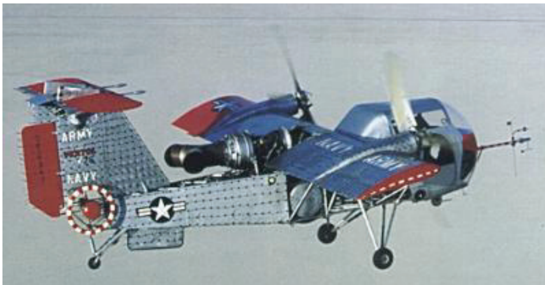
Fig. 3-96. The Vertol VZ-2 tiltwing proved more promising than the Ryan VZ-3. The first hovering flight of this 3,500-pound VTOL was on August 13, 1957, and the first full conversion back and forth from hover was made on July 15, 1958.
