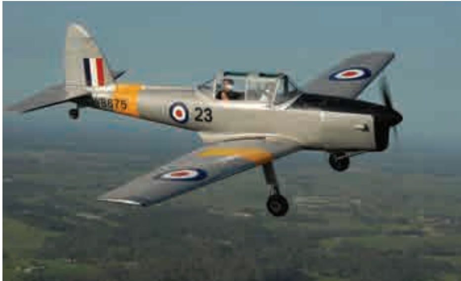
Fig. 3-158. The de Havilland DHC-1 Chipmunk was a small trainer that put the company back in the commercial business at the close of World War II. It was a monoplane rebirth of England's D.H. 82 Tiger Moth biplane. The brakes were hydraulic and the flaps were fabric-covered metal structures. Full-down flap setting was 30 degrees. De Havilland manufactured the wooden 78.8-inch-diameter propeller, which had an 18-degree pitch at the three-quarter radius [495, 500, 501, 604].
