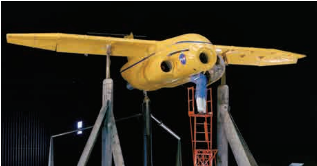
Fig. 3-70. The first-ever, large-scale augmentor wing test was made with only the compressors that provided BLC and jet flap blowing [447] (photo courtesy of Bill Warmbrodt, Ames Research Center).
