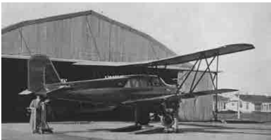
Fig. 3-157. The Glenn Curtiss Tanager was the outright winner of the Guggenheim Safe Aircraft Competition. It featured manually controlled flaps, floating ailerons, long-stroke rugged landing gear, and independently operated brakes. The propeller was fixed pitch [602, 603].
