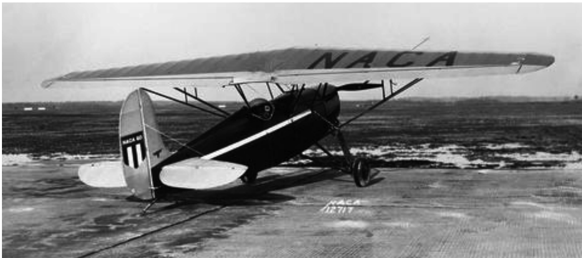
Fig. 1-8. The Langley modified Fairchild 22 had a 95-hp engine at 2,100 rpm. The wingspan was 31 feet with a chord of 4 feet 4 inches and an area of 132 square feet. The aspect ratio was 7.27, and the airfoil was a NACA 2415. The testing was conducted at a weight of 1,574 to 1,600 pounds (photo courtesy of Langley Memorial Aeronautical Laboratory).
