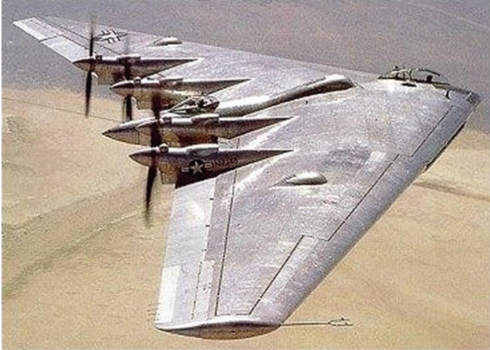
Fig. 2-33. Jack Northrop's XB-35 had a wingspan of 172 feet and a wing area of 4,000 square feet, which is an aspect ratio of 7.4. Four Pratt & Whitney R-4360 engines provided a total of 12,000 horsepower. The propellers were 15 feet, 1 inch in diameter and gave the 206,000-pound-gross-weight aircraft a maximum speed of about 340 knots (391 mph).
