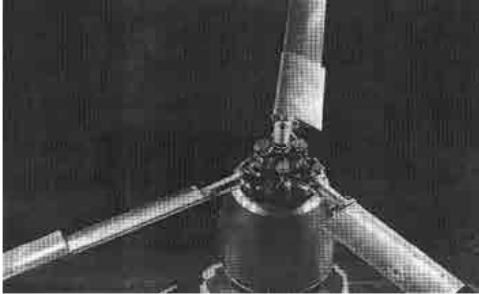
Fig. 2-11. The inboard segment of the 8-foot-diameter rotor blade was non-twisting . The rotor blades were untwisted, and the solidity was 0.119.
