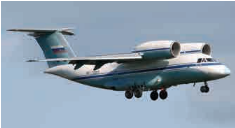
Fig. 3-197. The Antonov Design Bureau An-72 first flew in December 1977. Each Lotarev D-36 turbofan engine is rated at 14,330 pounds thrust. Wingspan is 84.75 feet and area is 969 square feet. At 58,420 pounds takeoff weight, the aircraft takes off in 3,280 feet. Maximum speed is about 410 knots. The aircraft is still in production.
