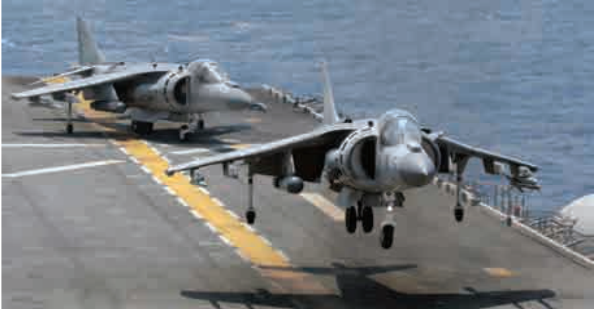
Fig. 1-25. The McDonnell/British Aerospace Harrier, a VTOL fighter powered with a gas turbine. To hover, the single engine directs all of its jet thrust downward.
