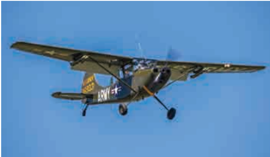
Fig. 3-159. The Cessna 305, the U.S. military L-19 (Bird Dog), replaced the Piper Cub L-4. With DOD Directive 4505 dated July 6, 1962, aircraft designations were changed, and the L-19 became the O-1 ("O" for observation). The brakes were mechanical. Full-down flap setting was 60 degrees. The McCauley 1A200/FM 9047, 7.5-foot-diameter propeller was fixed pitch. The blade angle at the 30-inch radius ( r/R = 2/3 ) was 14 degrees. Minimum ground run distance was obtained with power-off landing. At a gross weight of 2,200 pounds and touchdown airspeed of 43 knots, distance was about 320 feet [576, 605-607].
