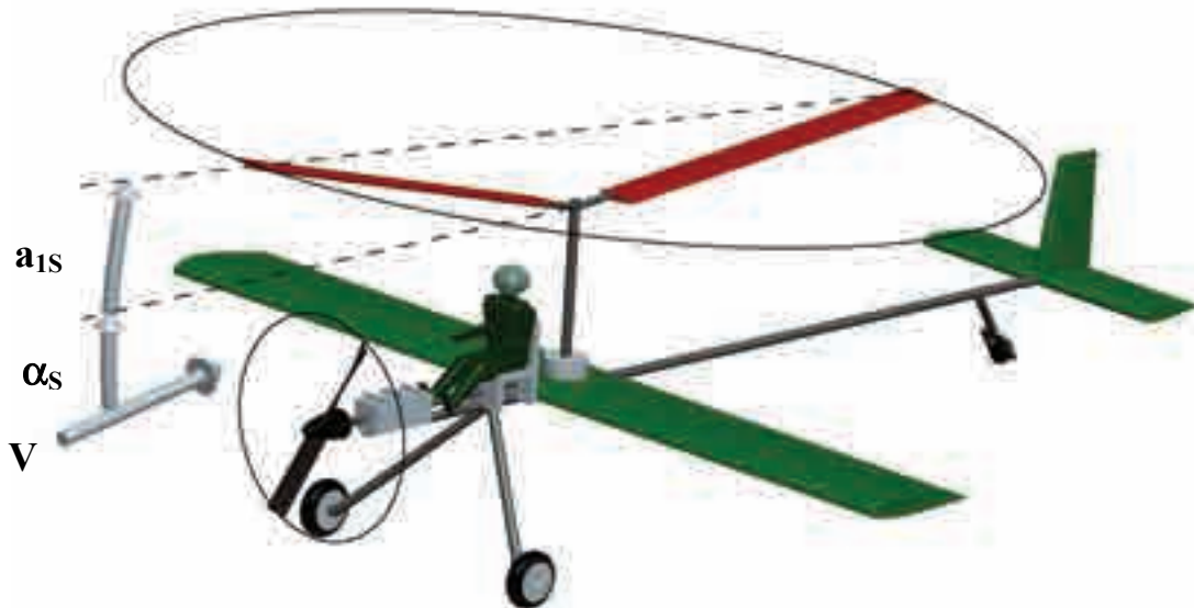
Fig. D-1. The simple elements of compound aircraft. Tail rotor not shown for clarity. Rendition by Gerardo Nunez from author’s sketch.
