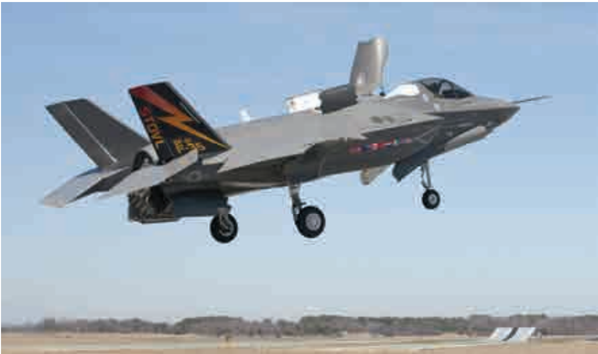
Fig. 1-30. The Joint Strike Fighter, the F-35, is a slightly compromised V/STOL called a STOVL, which stands for Short Takeoff and Vertical Landing. The approach defines the mission takeoff gross weight based on a STOL takeoff rather than a vertical takeoff. After fuel is burned off, a vertical landing and takeoff is easily accomplished.
