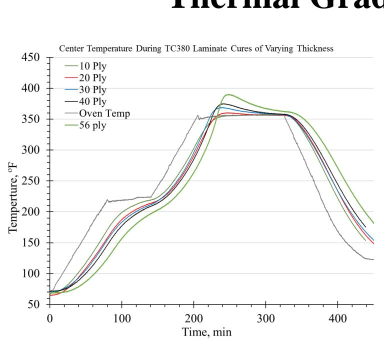
Thermal lag in center of composite increase significantly with large number of plies, going from 150 minutes to reach 225 F in a 10 ply laminate to nearly 180 minutes to reach 225 F in a 56 ply laminate
