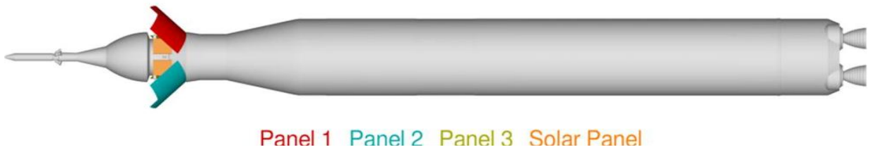
Figure 1. Side view of SLS Center Body geometry with panels open at 45° on hinge.
