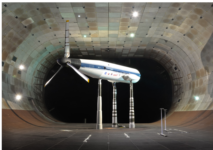
Fig. 1 TTR/699 installed in the USAF NFAC 40- by 80-Foot wind tunnel test section.
