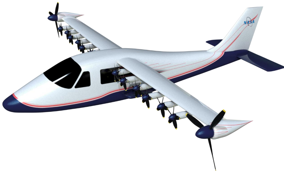
Figure 1. Rendering of SCEPTOR vehicle concept. 2
