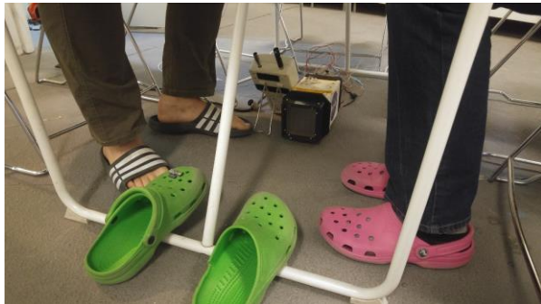
Figure 14: OPC and SFS location underneath the table of the upstairs work area for Test #8 to measure ambient dust conditions in the residential sections of the habitable volume.
