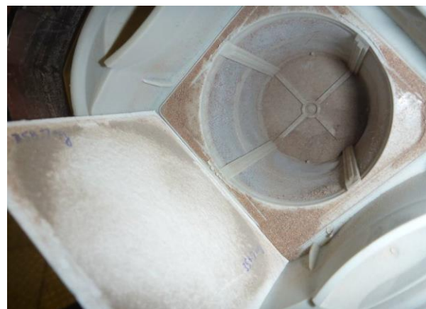
Figure 9: Vacuum filter with additional NASA filter after EVA #14 airlock cleaning.
