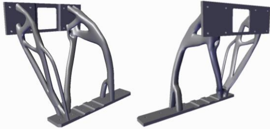
Fig. 15: Topological optimised single-piece design of the supporting bracket for the upper thruster pod in Aluminium alloy (option 2)
