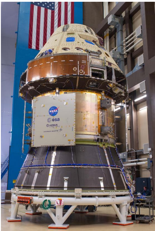
Fig. 3: Engineering model of the Orion stack (from bottom-up): SA / ESM / CMA/ CM
