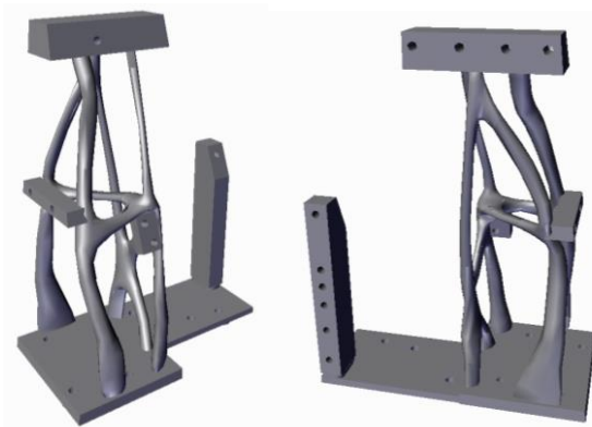
Fig. 20: Design of the third “Rusty Tower” bracket obtained by topology optimisation
