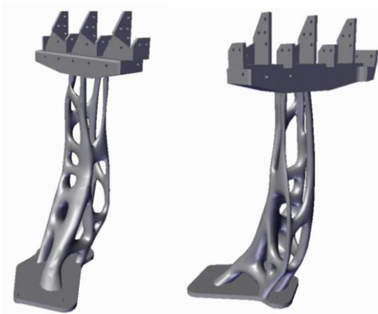
Fig. 19: Design of the second “Rusty Tower” bracket obtained by topology optimisation
