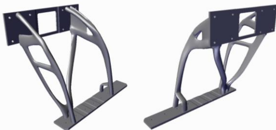
Fig. 16: Topological optimised single-piece design of the supporting bracket for the upper thruster pod in Titanium alloy (option 3)
