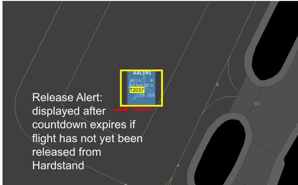
Figure 4.8. Alert to Release From Hardstand.
