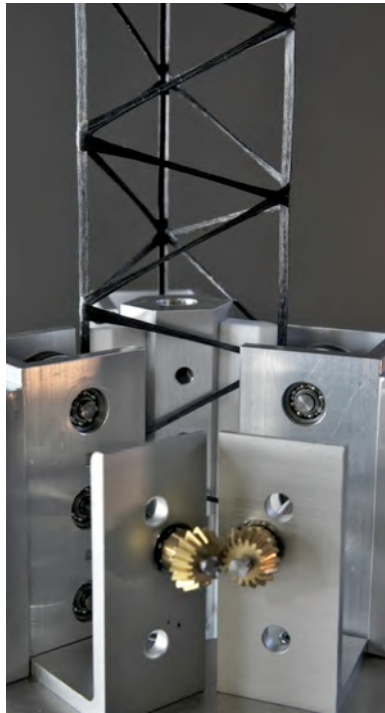
Figure 5. Close-up of the carbon-fiber truss exiting the Trusselator prototype.
