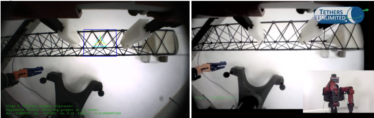
Figure 48. Robot identifying truss grasping point and then capturing it with the final gripper design.
