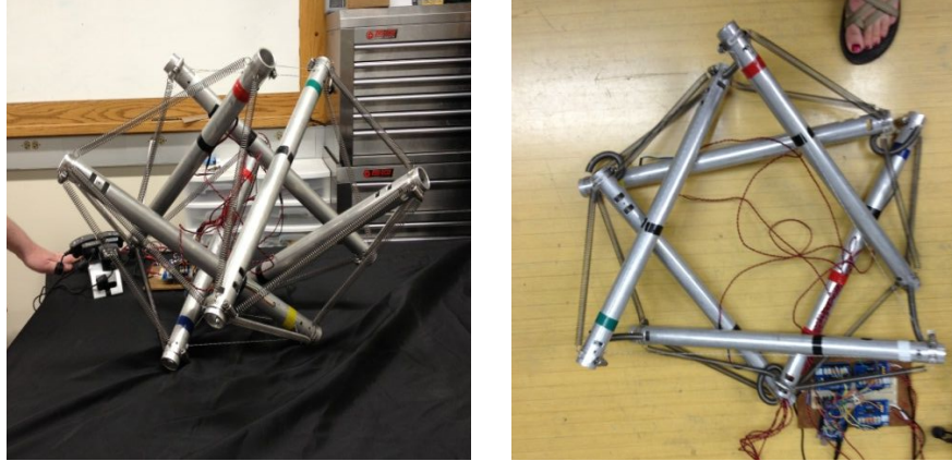
Figure 44: Tensegrity under Star Elongation Method of Collapse.
