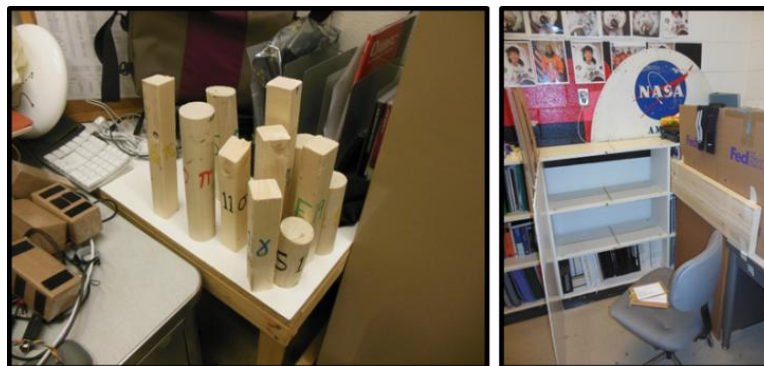
Figure 4-49: BUFF Test Experimental Setup. The bookshelf was divided into 12 regions, with each of the three shelves containing four quadrants
