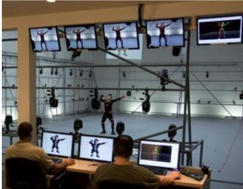
Figure 5-3 – Example optical motion tracking setup and infrastructure. (www.creativeplanetnetwork.com)
