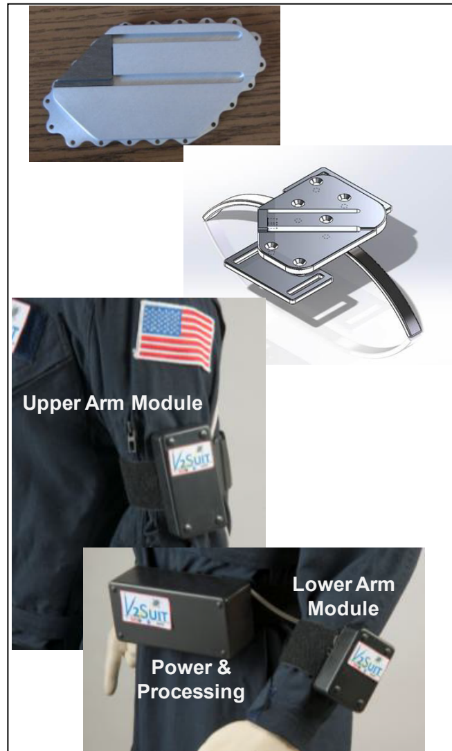
Figure 5-5 – Top: Contoured plate (lace-in and double-strap versions) (courtesy of David Clark Company Inc.), Bottom: Concept of V2Suit module placement.
