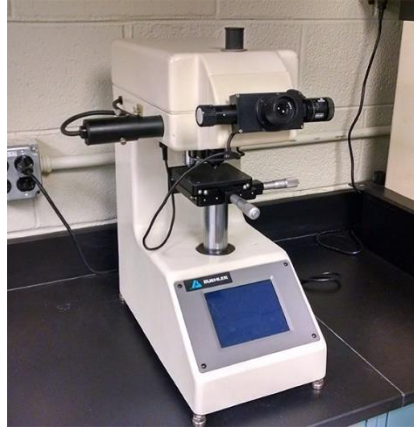
Figure 4: Buehler Model 1600 hardness tester with Vickers hardness indentation tip.
