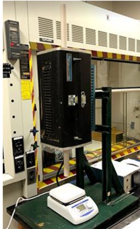
Figure 6: Vertical tube furnace configuration used to determine thermal shock temperature change for asteroid regolith simulant.
