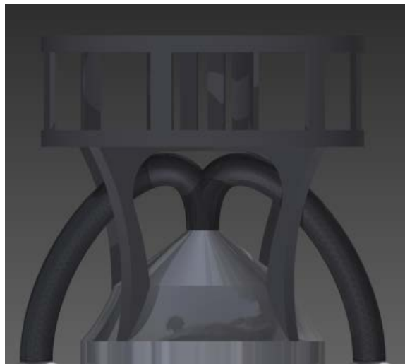
Figure 19: Artistic rendering of the 6U toroidal cage designed to house the instrumentation payload
