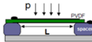
Figure 24 Piezoelectric sensor construction (image credit: Xerox PARC)
