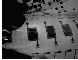
Figure 23 - Western Michigan University Printed Humidity Sensor
