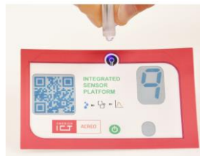
Figure 26 Acreo low-cost, printed, UV sensor system
