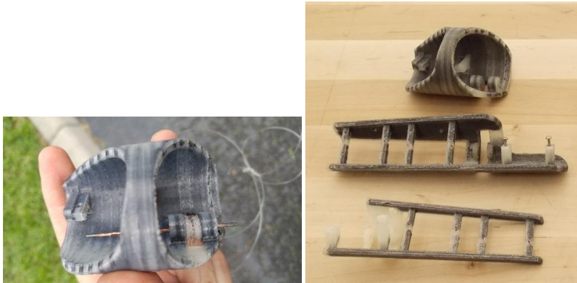
Figure 10. Cable connection/release mechanism with servo-driven linear pin (left); Subsequent versions of the cable release mechanism shown without servos/pins (right)
