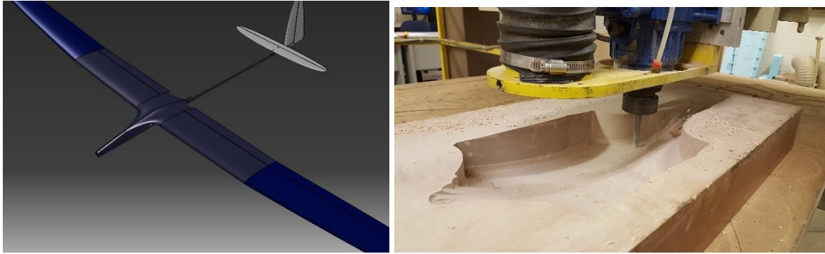
Figure 13. MANTA center-section in gray with MAXA wing tips/tail (left); manufacturing of tool for MANTA (right)
