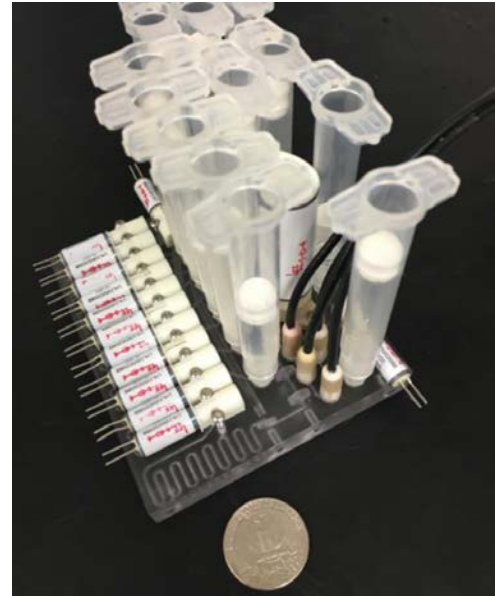
Figure 46 An example of microfluidics chip. a: 3D printed MicroFIA manifold, b: assembled MicroFIA system. Images taken from (Kehl, et al., 2016).
