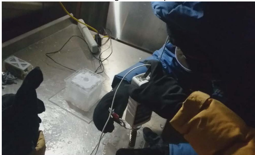
Figure 52 - Required normal force to begin insertion of the ice screw was measured with a force gauge by Aaron Curtis. About 6\text{ N} appeared to be the minimum required force.
