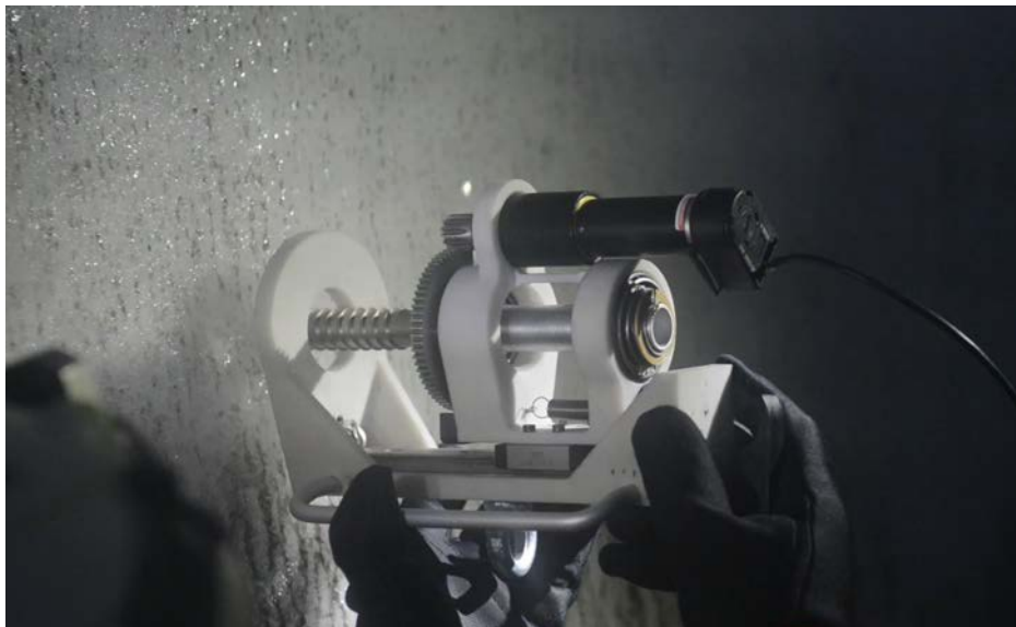
Figure 3. Test of a prototyped ice screw end effector in Helo Cave, a fumarolic ice cave on Erebus volcano in Antarctica.
