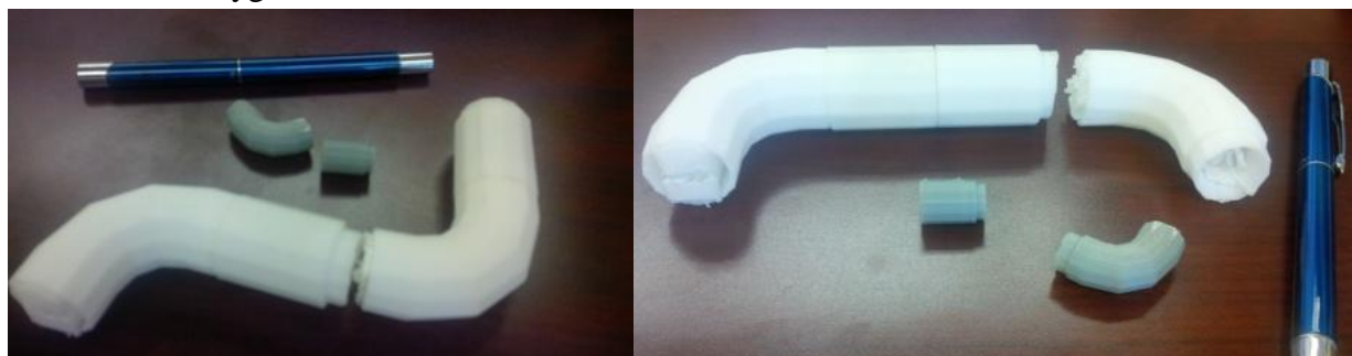
Figure 10. "Lego-like" 3D printed device module that can be individually designed and configured.
