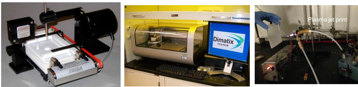
Figure 17. Thin film deposition experiment set ups at ARC labs from left to right: Langmuir Blodgett monolayer deposition trough, piezoelectric nano-jet printer (Dimatix) and a home-made plasma jet printing
