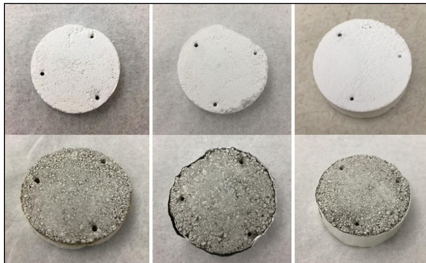
Figure 2.9-1. Silver-coated BaF 2 samples showing a grey color.
