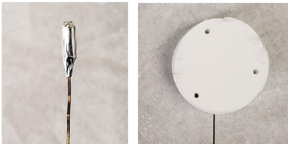
Figure 3.2.3-2. A temperature sensor wrapped in silver and then installed between two Y_2O_3 rigid samples.
