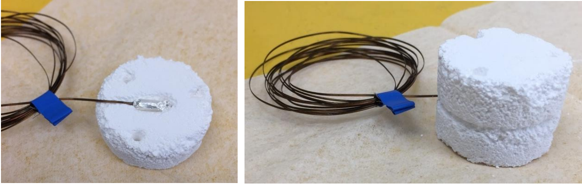
Figure 3.2.4-1. Barium Fluoride sample with the temperature sensor wrapped in silver foil. One image shows the temperature sensor nestled in a cutout in the center of a rigid barium fluoride disk and the other images shows a second barium fluoride disk placed on the first one to form a test sample where the temperature sensor is in the center of the sample.
