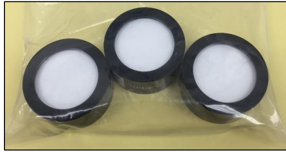
Figure 2.1.1-1. Typical powder test samples consist of a 1-inch diameter cylindrical holder, allowing two windows to sandwich the powder. This assembly permits reflectance and transmission measurements of the powder.
