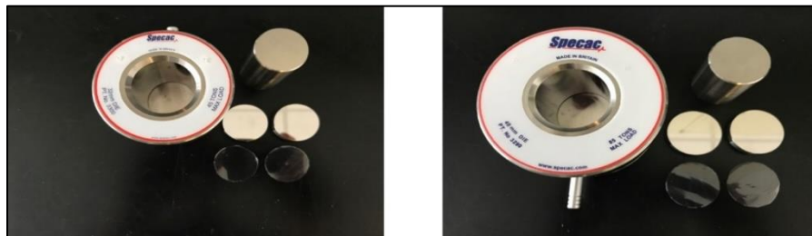
Figure 2.1.2-3. Specac 32 mm and 40 mm diameter steel molds and assorted dies or plungers used in a hydraulic press to compact the barium fluoride powder.
