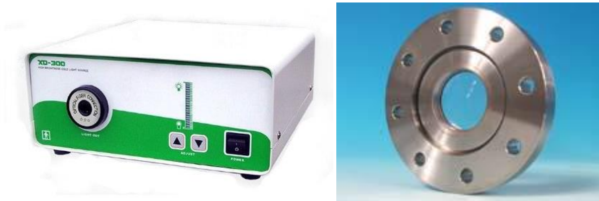
Figure 3.2.1-2. A Xenon Lamp was used as a solar simulator and a sapphire viewport was used to seal the vacuum chamber, but allow the radiation from the Xenon lamp to enter.
