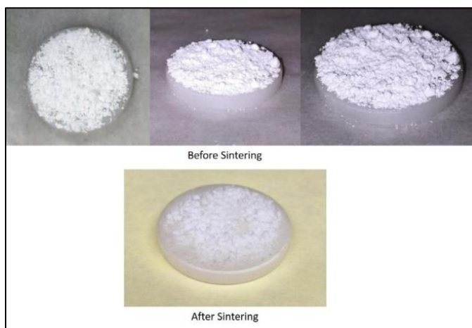
Figure 2.1.2-1. Barium fluoride powder sintering example showing three images of barium fluoride powder spread on top of a one-inch diameter, barium fluoride window labelled “before sintering” and an image of sintered barium fluoride on a barium fluoride window labelled “after sintering”.
