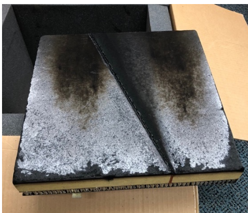
Figure 21. Post-test panel of MSL-era PICA coated with NuSil shows persistent glassy silica residue.
