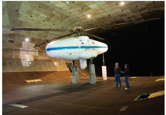
Figure A-50. UH-60A rotor in the NFAC 40- by 80-Foot Wind Tunnel (courtesy of NASA Ames Research Center).
