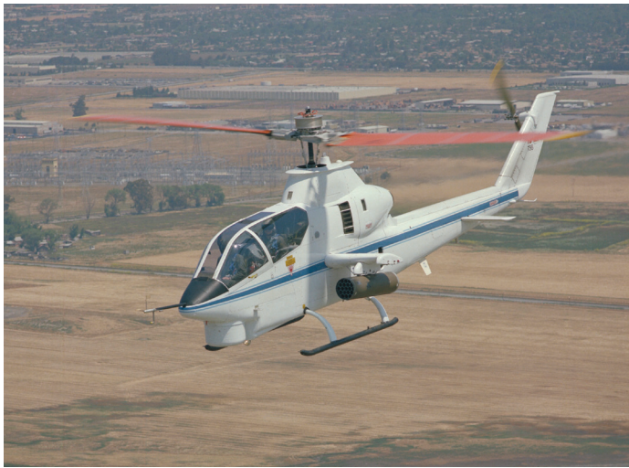
Figure A-39. AH-1G/TAAT airloads test aircraft (courtesy of NASA Ames Research Center).
