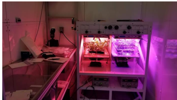
Figure 2 (above). The growth chamber contained a setup similar to flight, with the lighting treatments grown in proximity of one another. Figure 3 (below). Harvesting mizuna on 28 DAP.
