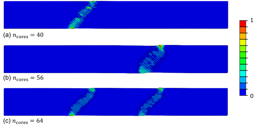
Figure 9. Matrix cracking damage variable showing three different cracking patterns for three different number of cores.
