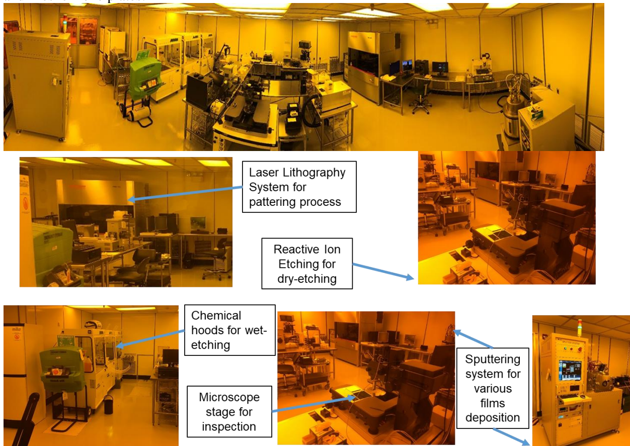
Figure 3. Photo of the ISO5 Optical Cleanroom and housed instruments at NASA Langley Research Center
