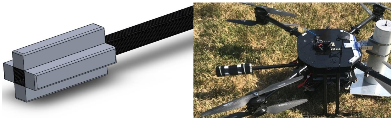
Figure 17. CAD drawing of the counterbalance (left) and the photo of the counterbalance on payload (right).
