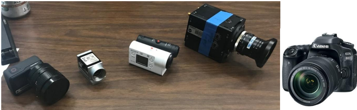
Figure 32. Photos of candidate cameras for the telescope payload. Left to right shows GoPro HERO6, Basler acA2500-14gm, Sony FDR-X3000, IDT NX4 Air, and Canon EOS 80D
