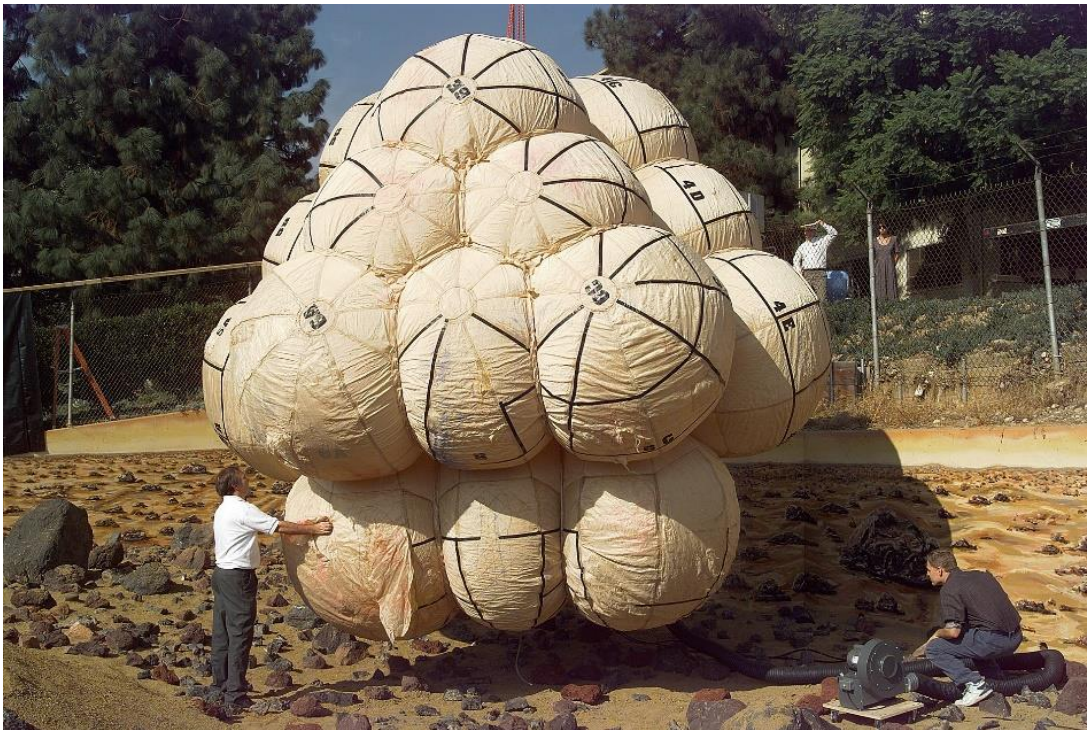
Figure 4. Mars Pathfinder's large, multi-lobed air bags are inflated and tested in 1995 5 .
