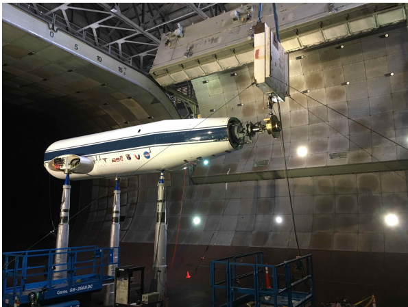
Figure 2. Shake test setup – vertical shaking at the hub – 0 deg yaw (airplane mode)
