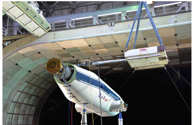
Figure 5. Shake test setup – lateral shaking at forward lifting lug – 0 deg yaw (airplane mode)
