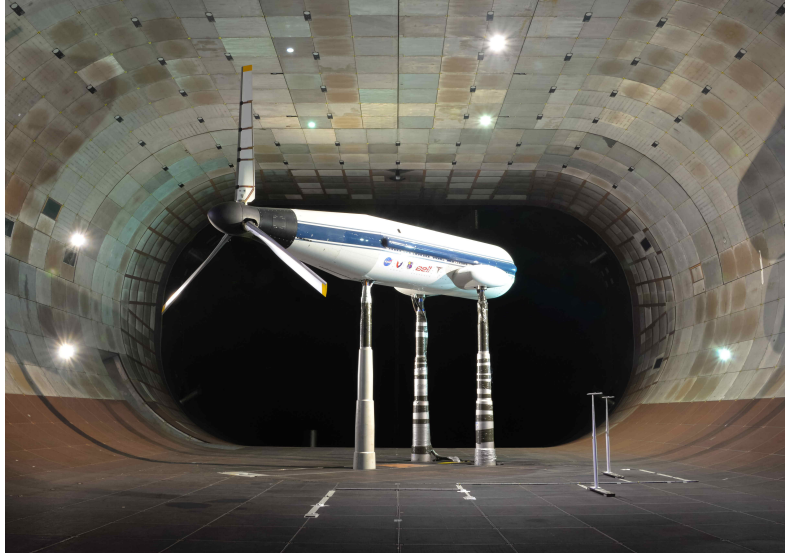
Figure 1. Tiltrotor Test Rig (TTR) installed with the 609 rotor in the 40- by 80-ft test section of the National Full-scale Aerodynamics Complex – 45 deg yaw (conversion mode)
