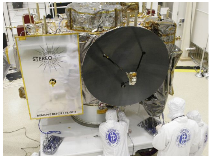
Figure 10. STEREO High Gain Antenna 1.2m parabolic dish
