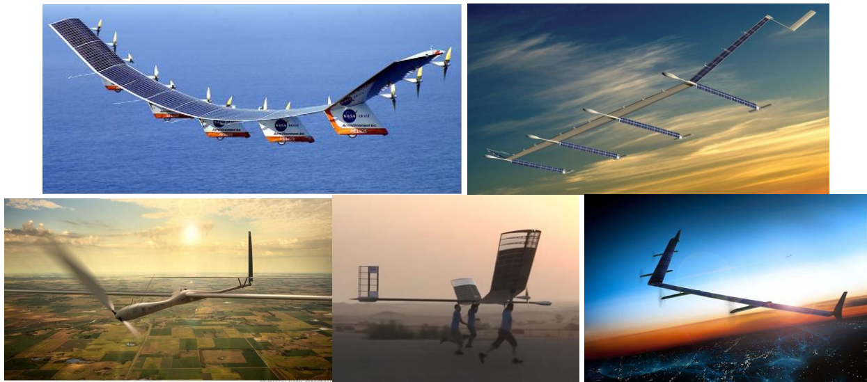
Figure 1. Stratospheric solar aircraft development efforts (top: AeroVironment's Helios, Boeing's SolarEagle; bottom: Google's Solara, Airbus' Zephyr, Facebook's Aquila)
