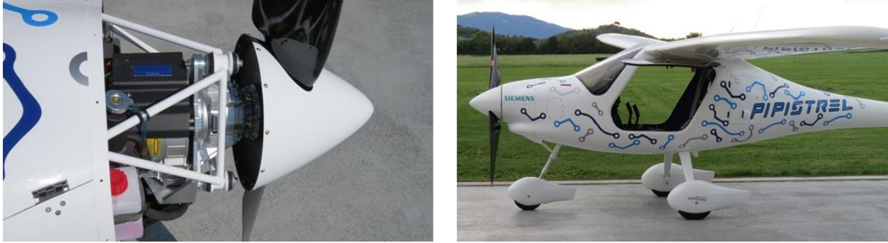
Figure 8. Pipestral's WattsUP Prototype with propeller that can extract wind energy as a turbine
