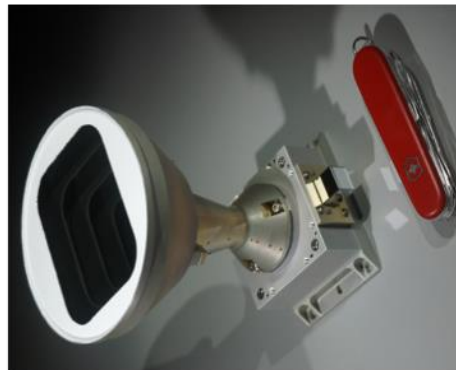
Figure 5. VisCAM Camera, a COTS low mass, volume, and power Malin Space Science Systems Camera with optics modified to allow 8 meter resolution at 300 km, as described in the text.
