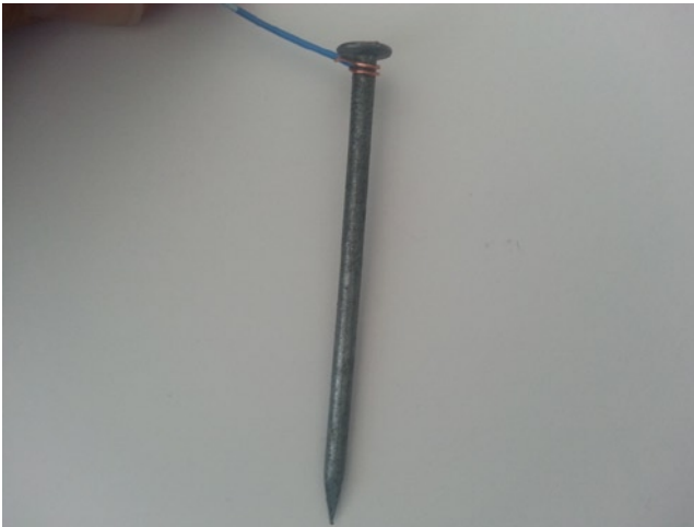
Figure 8-4. Wrapping the wire around the nail's head
