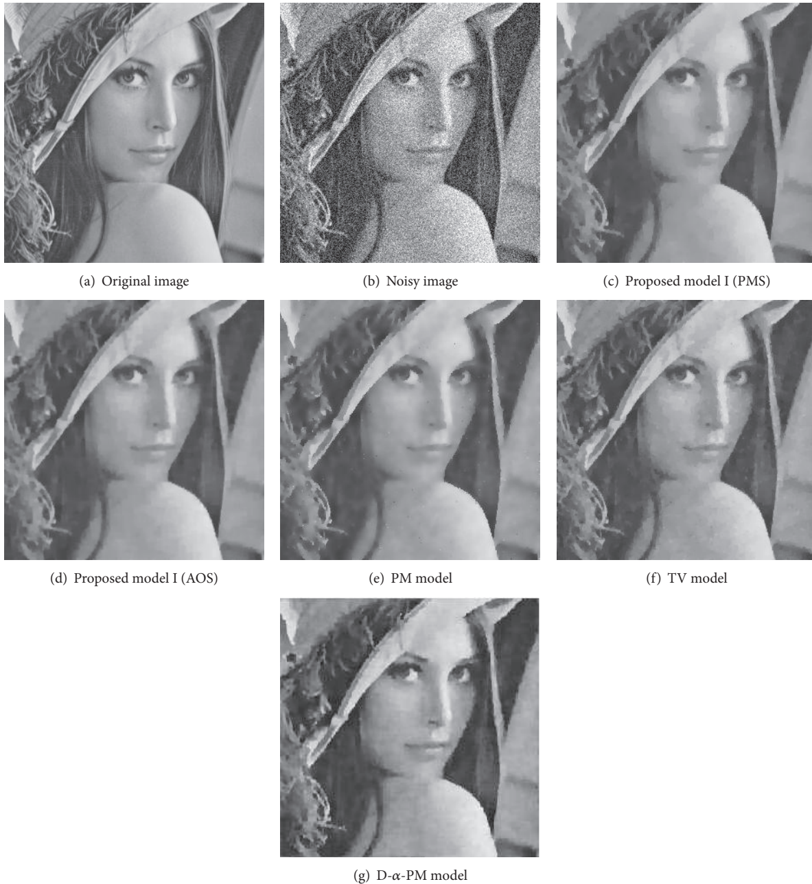
FIGURE 3: Lena image ( 300 \times 300 ). (a) Original image. (b) Noisy image corrupted by Gaussian noise for \sigma = 30 . (c) Our algorithm by PMS; \tau = 0.2 (122 steps). (d) Our algorithm by AOS scheme; \tau = 2 (7 steps). (e) PM method; K = 12 and \tau = 0.25 (60 steps). (f) TV method; \tau = 0.2 (149 steps). (g) D- \alpha -PM method; \sigma_1 = 0.5 , \sigma = 30 , \tau = 2 , and K = 4 (13 steps).
