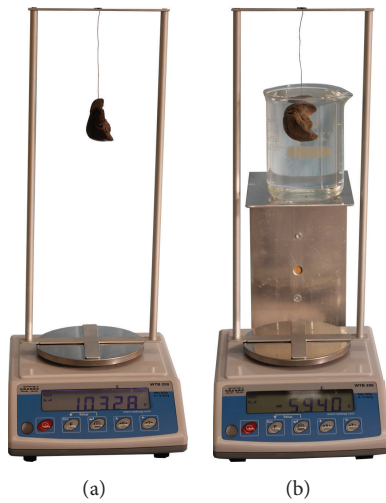
FIGURE 1: A double weighing procedure to obtain the weight of the liver in air (a) and distilled water (b).
