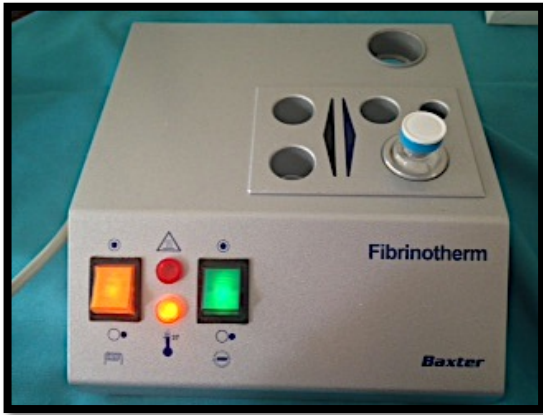
Figure 2.6: Turning on the green switch to activate the magnetic stirring well
