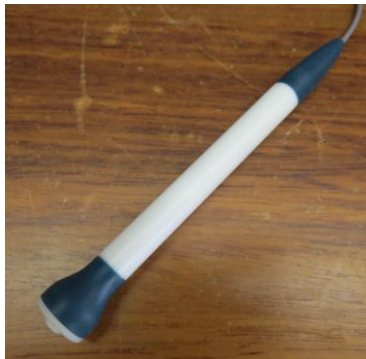
Figure 3.1 A SphygmoCor device coupled with an applanation tonometer (panel A) which was used to determine aortic haemodynamics. Panel B illustrates the applanation tonometer used to detect the pressure waveforms.
