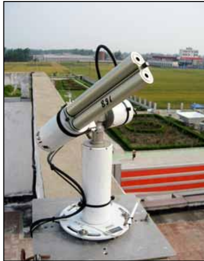
Figure 3.9: The CIMEL Sun Photometer used as part of AERONET is used in the calibration of the hazemeters ( www.arm.gov/instruments/csphot ).
