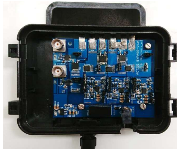
222 223 Fig. 5. Rear side photovoltaic module junction box containing 224 three bypass circuits. In the periphery the board contains 225 additional circuits for sensing purposes. 226
