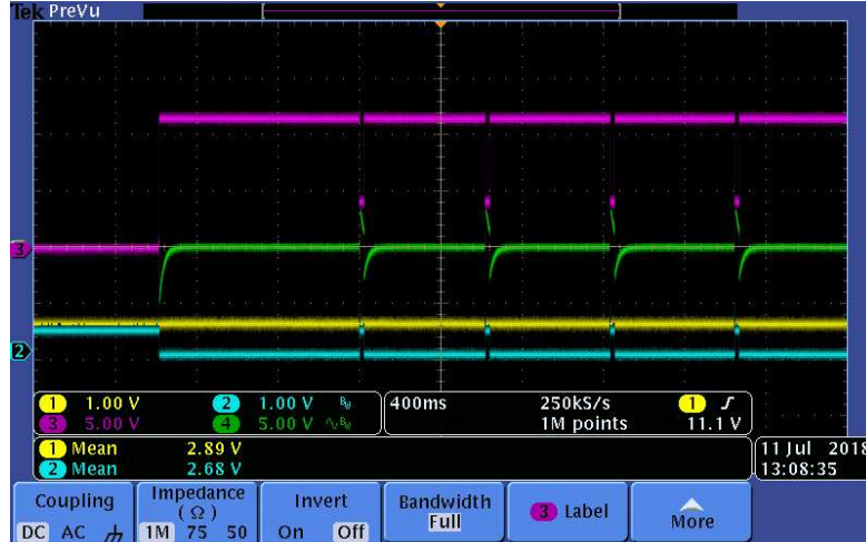
Fig. 12. Digital oscilloscope view of electrical signals during a bypass event.
