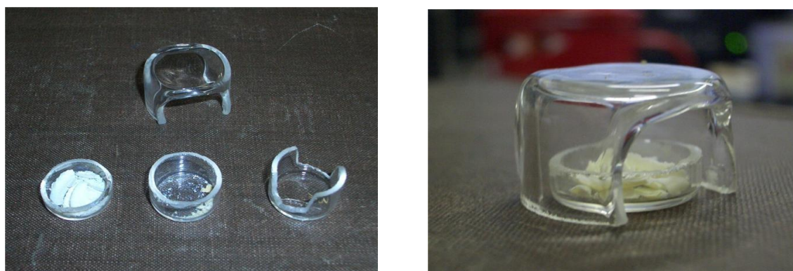
Figure 5. (a) The sample pans and the cover (b) Assembled pan and cover
