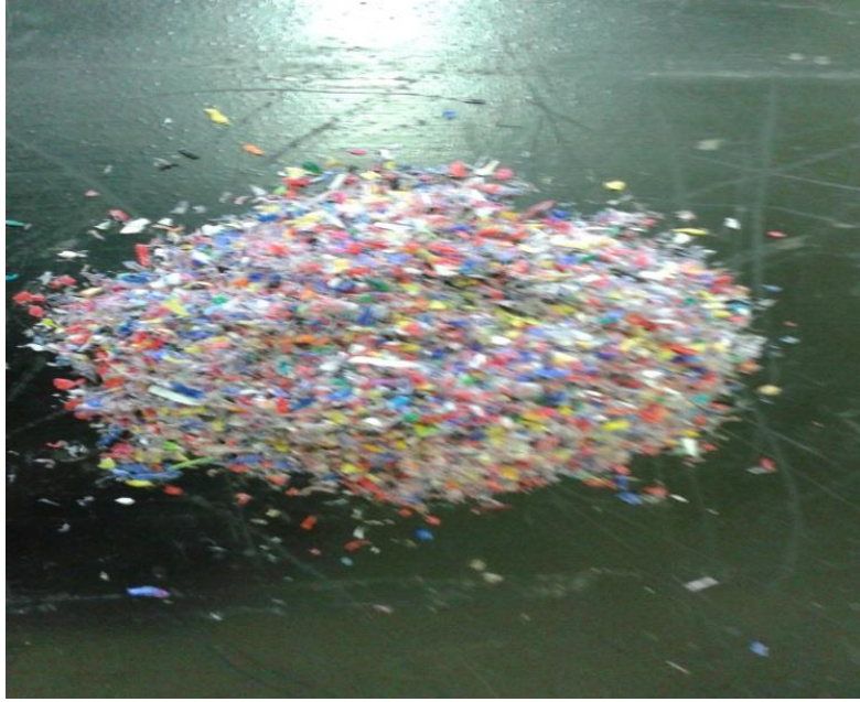
Figure 4.7 Milled and sieved polypropylene waste plastic
