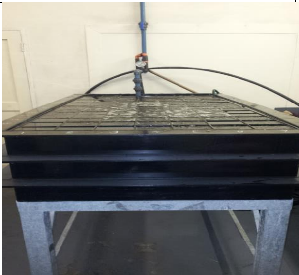
Plate 3. 11 : Installed water stability system
