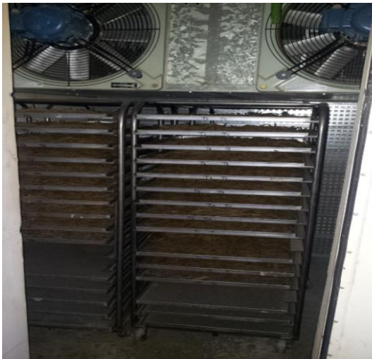
An air dryer chamber
