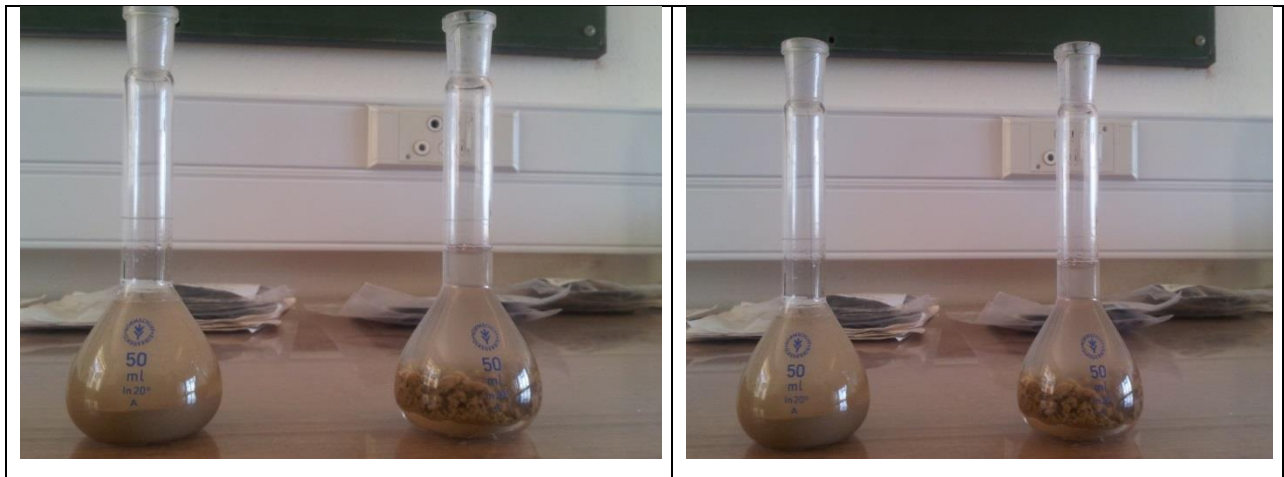
Plate 4.5 : Clay mineral used for the study (From L-R: Natural bentonite, acid-activated bentonite clay)
