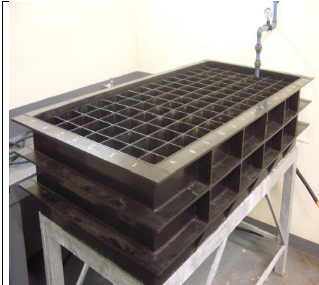
Plate 3. 9 : Installed water stability grid
