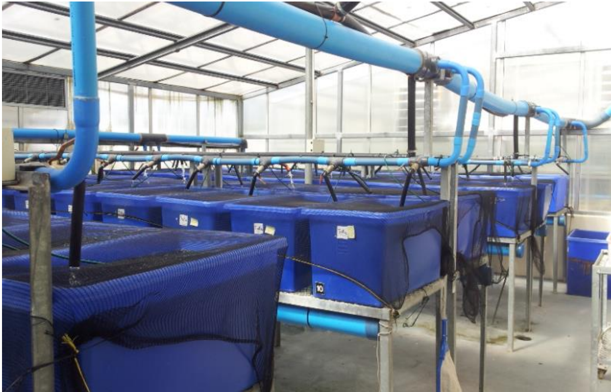
Plate 4. 4 : Recirculating aquatic system used during the experiment, incorporating 88 rectangular plastic tanks
