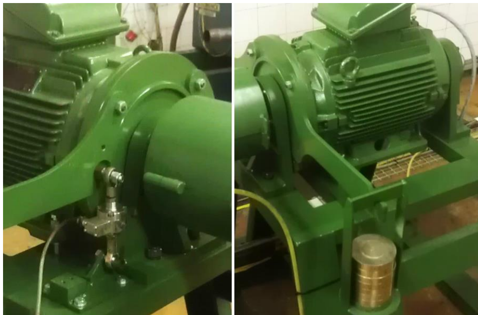
Figure 13: Load cell (left), calibration arms and weight tray (right)
