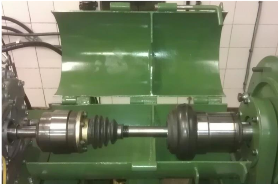
Figure 14: Driveshaft and safety guard
