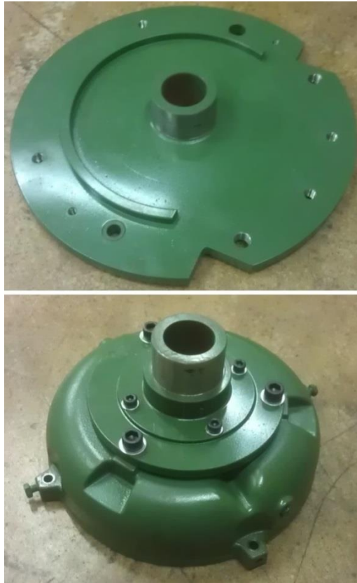
Figure 11: Drive end flange (top) & non-drive end flange (bottom)
