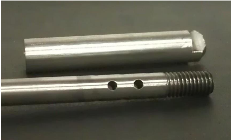
Figure 19: Designed smoke probe (bottom) and stainless steel cap (top)
