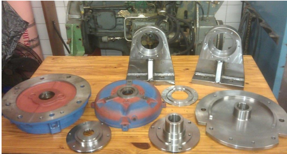
Figure 12: Machined dynamometer components prior to being painted
