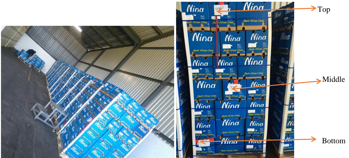
Figure 24: Ambient and fruit pulp iButtons® location from pack house to cold store
