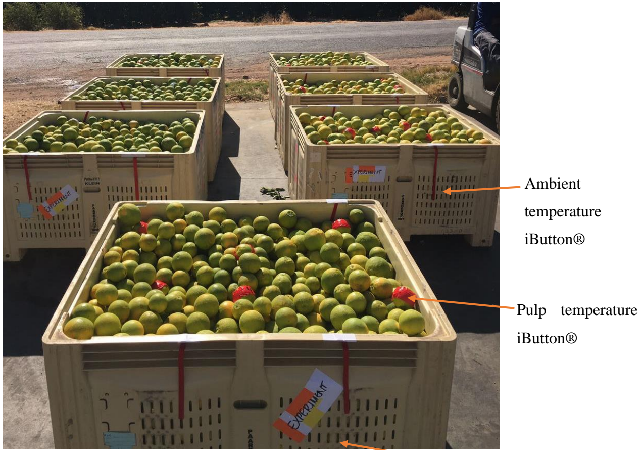
Figure 23: Pulp and ambient iButtons® in bins at the orchard
