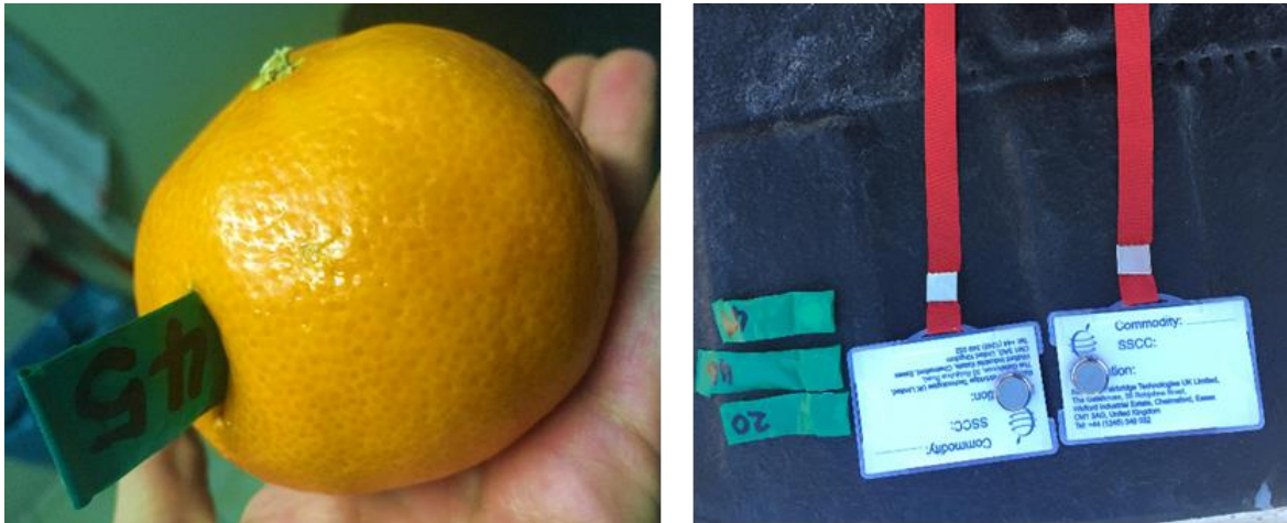
Figure 22: Illustration of iButtons® probed inside a navel orange and ambient recording iButtons® with a red string attached.
