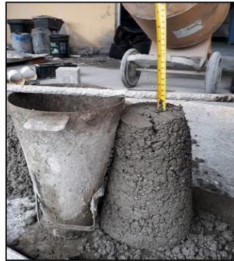
Fig. 4. Slump cone for workability of concrete.
